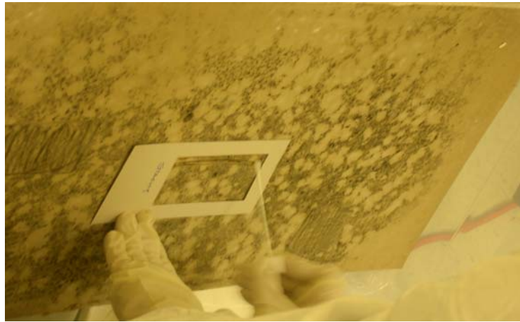
Figure 4. Sampling of viable Stachybotrys chartarum
