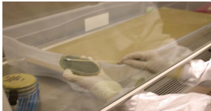
Figure 2. Application of harvest cultures onto drywall
