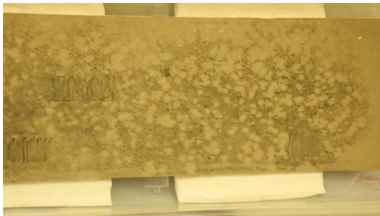
Figure 5. Drywall with Stachybotrys chartarum post ozone treatment
